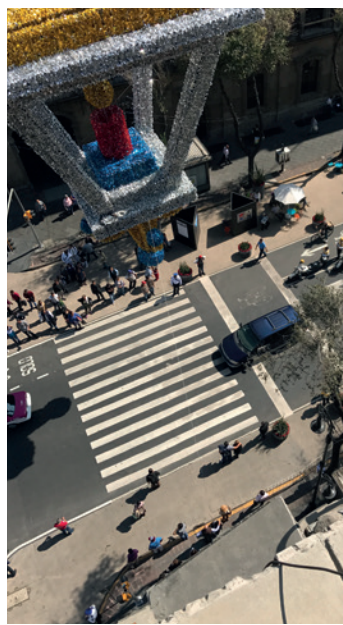
Paint is used to widen sidewalks and add a mid-block crossing in Mexico City
